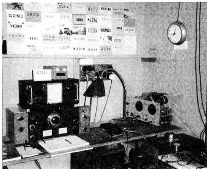
40 years on. Old soldiers need not fade away if kept going with injections of new bits and pieces. A January 1984 photograph of the station of George Hook, G2CIL, features two long lasting items of wartime equipment: a modified HRO (re-valved with EF92s etc) and a vfo/45W rig built around the once-popular TU5B tuning units. George shows he ain't agin modern lc devices with an SL6600 for fm reception!
